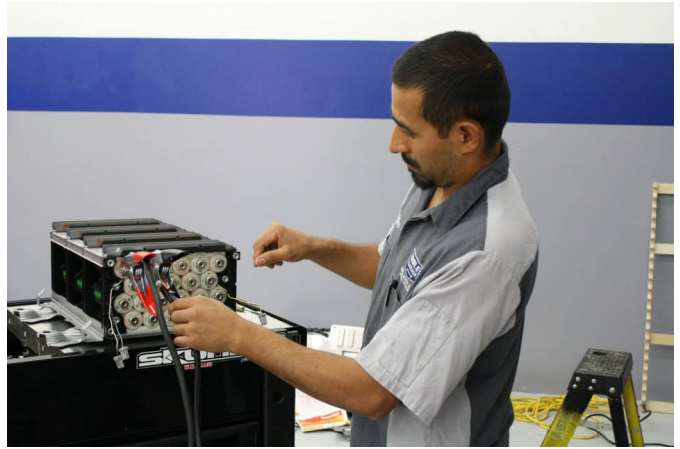
Staff performing test on hybrid vehicle battery.
