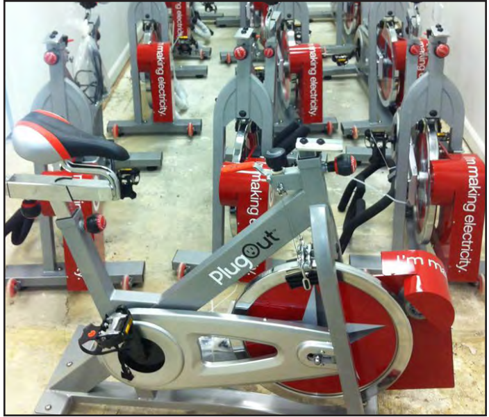
These gym bikes generate electricity for the business when used by customers, making Elevated Fitness carbon neutral.
