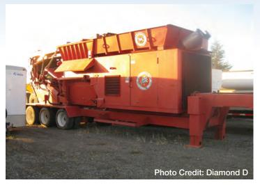
Diamond D uses a Morbark "Predator" Shredder to break large material into eight inch or smaller pieces, reducing the space needed to house this material in landfills.
