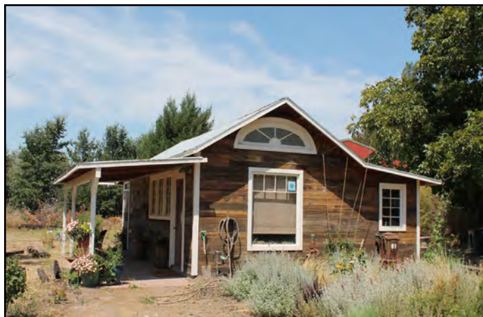
The porch is designed to keep heat from the afternoon sun off the studio
